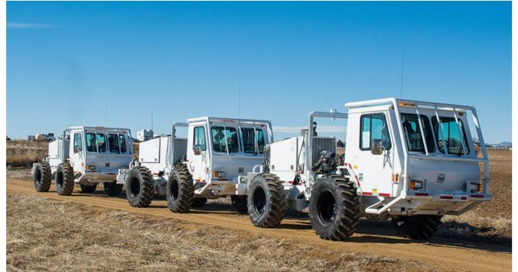
*Seismic trucks used in a 3-D seismic survey*
